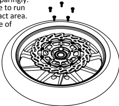
\*\*When a turning direction is marked on the disc, make sure to match the direction with the turning direction of the wheel.
